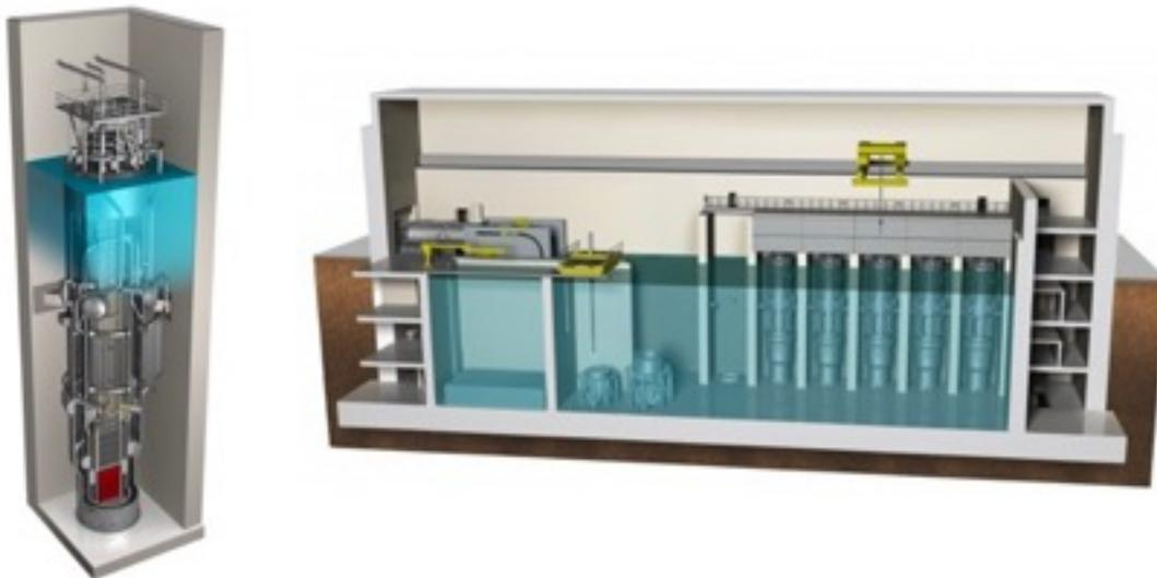
Figure A-3 VOYGR™ nuclear power module (left) and arrangement in reactor building (right)
