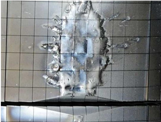
JET runaway electrons damage. https://www.iter.org/newsline/-/2234
