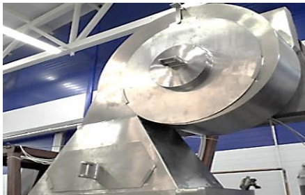
Argon cooling and recirculation unit
