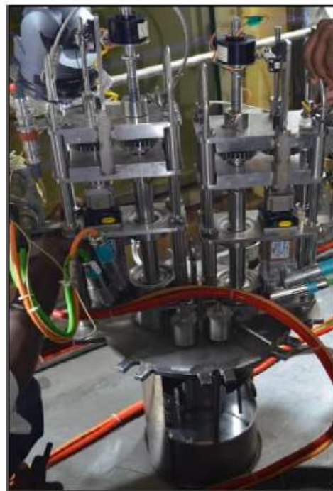
Fig. 15. Photograph of electrode assembly with top flange and reaction crucible.
