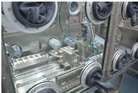
FIG.7 Machine vision based slug inspection
