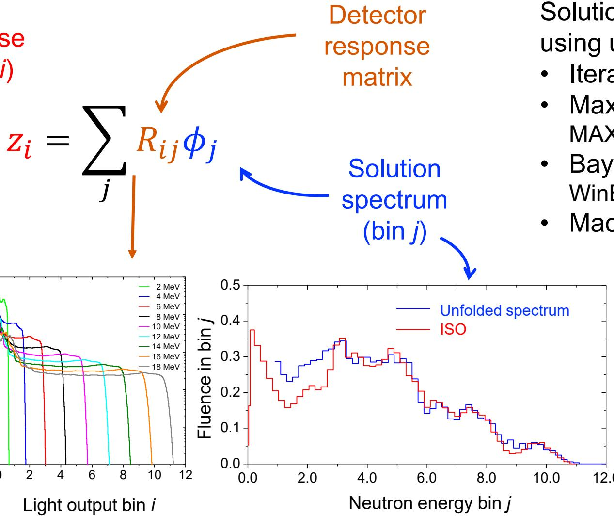
Solution spectrum obtained using unfolding algorithm:
