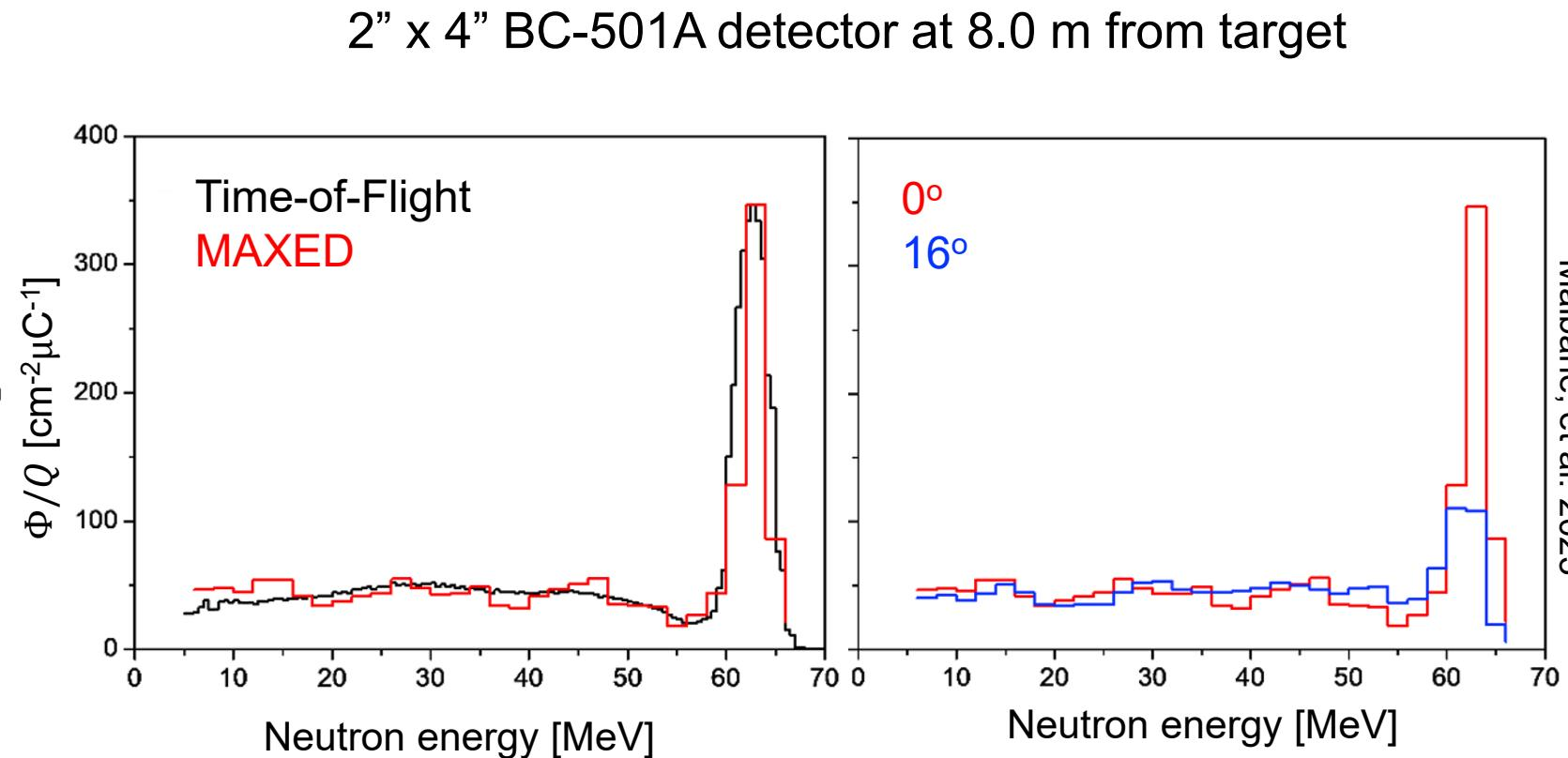
Neutron energy spectra corrected for detector efficiency
