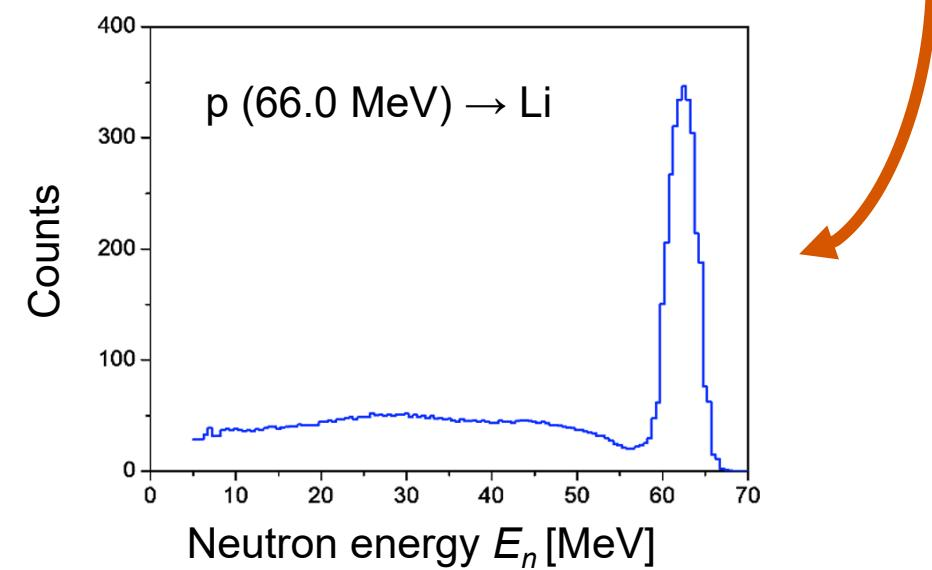
**Measurements of neutron energy spectrum (via Time-of-Flight)
