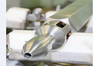
BN-600 Fuel assemblies with (U Pu) N Courtesy of VNIINM, Russia
