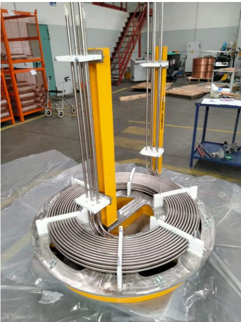
SGTS spiral-tube bank (test operations before assembly)
