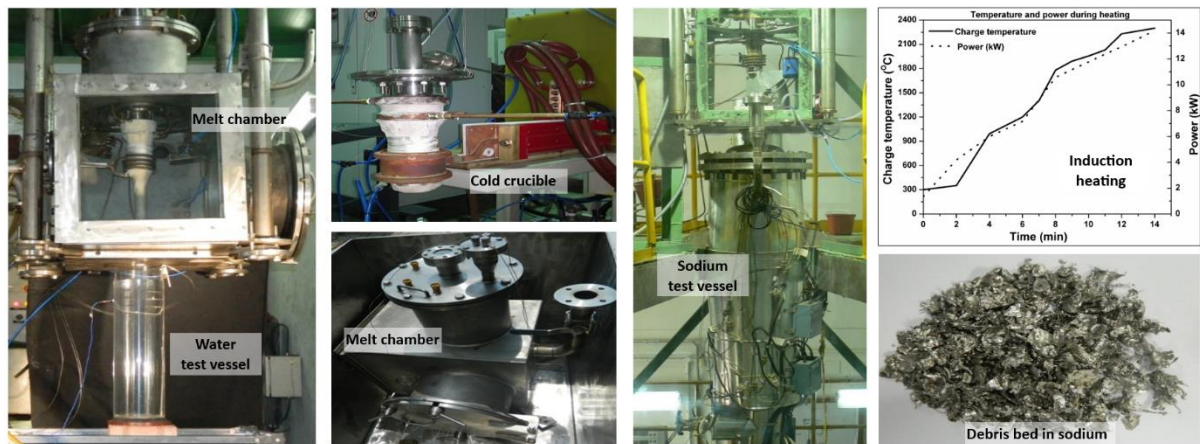
FIG.1 Experimental setup with cold crucible and melt chamber at SOFI facility
