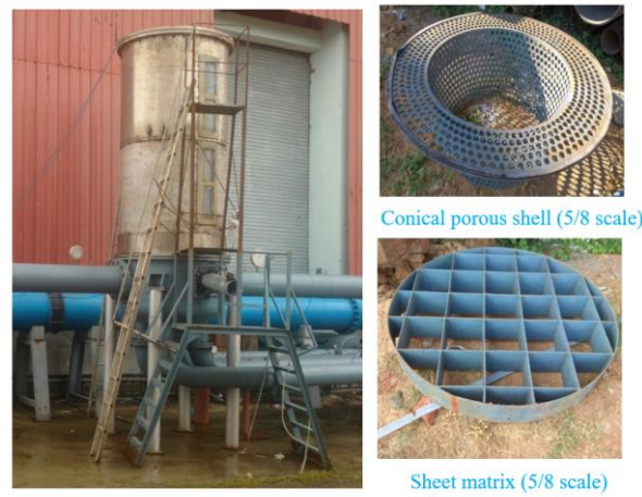
FIG. 4. 5/8 scale model of surge tank and gas entrainment mitigation devices
