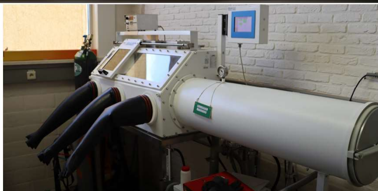
TIG - SPOT WELDINGS IN THE GLOVE BOX
