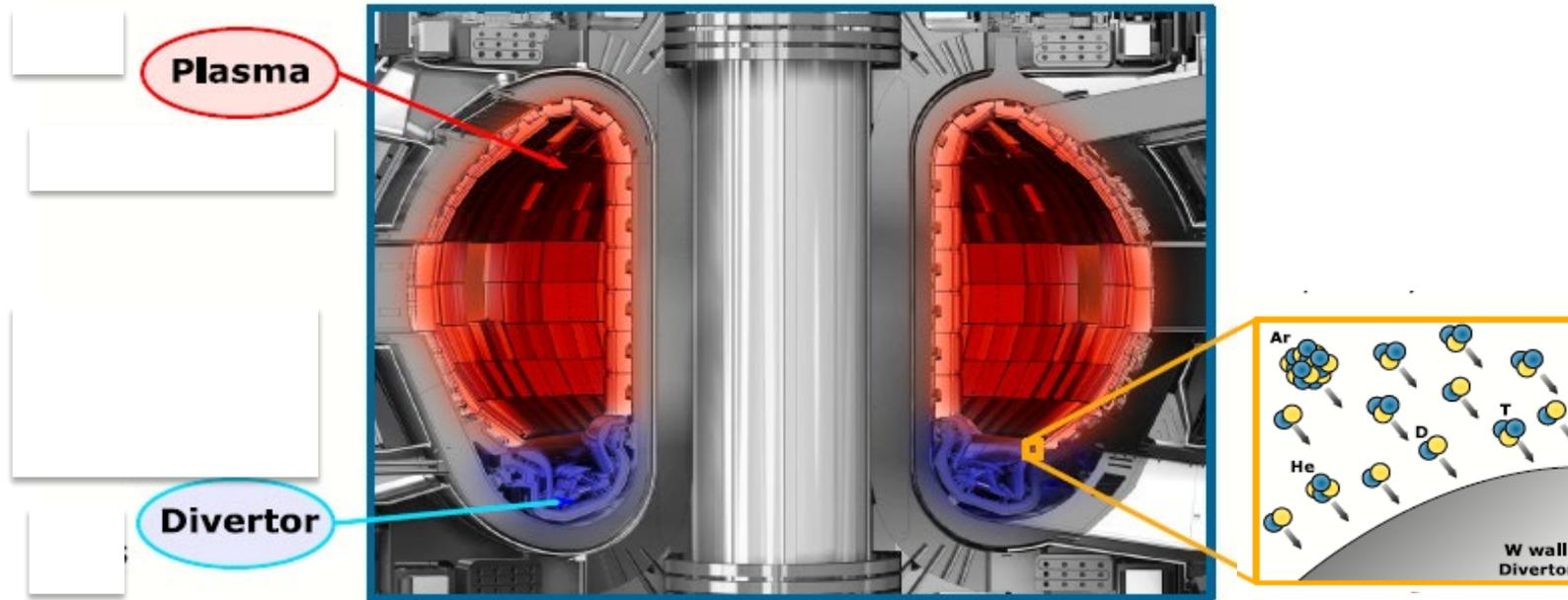
TOKAMAK reactor concept [2]
