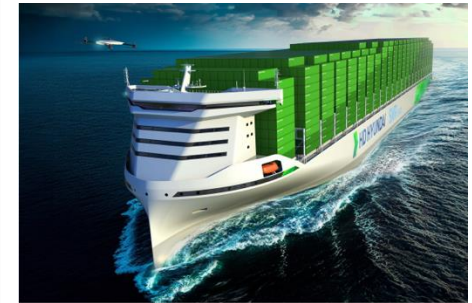
A rendering of a 15,000 TEU-class SMR-powered container ship (Image: HD KSOE)
