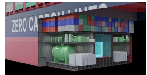
A rendering of a 15,000 TEU-class SMR-powered container ship (Image: HD KSOE)
