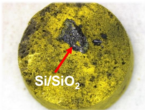
After dissolution of U_3Si_2 in MoO_3
