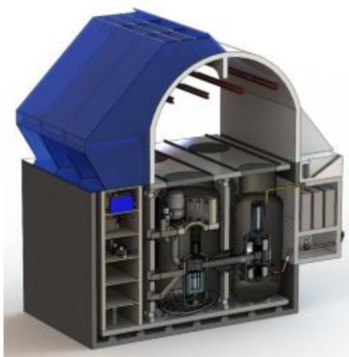
Elevation view of EM 2 modular building element employing two modules on a single seismically isolated platform
