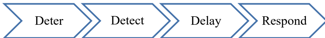
FIG. 2. Security system functions.
