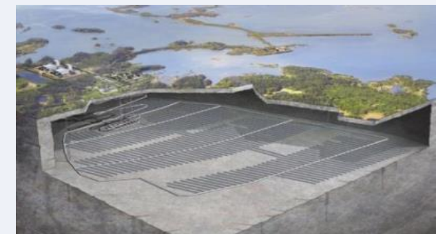
Spent Fuel Repository at Osthhammar (Courtesy of SKB)
