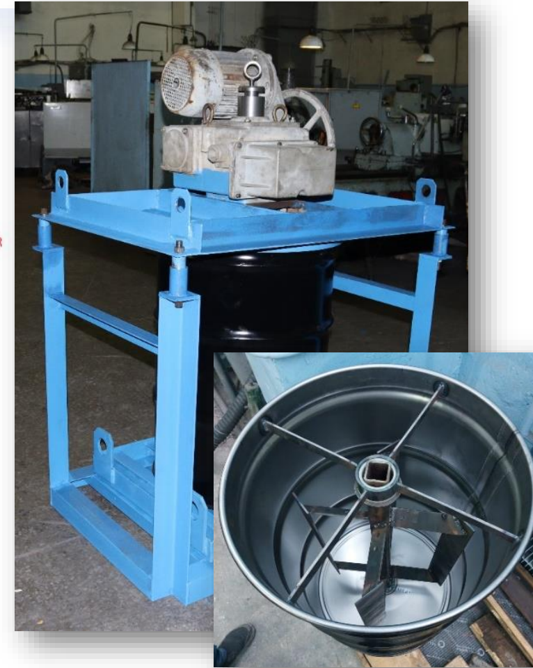
55-gallon drum from Skolnik CQ5508 Built-in mixer from NNC RK
