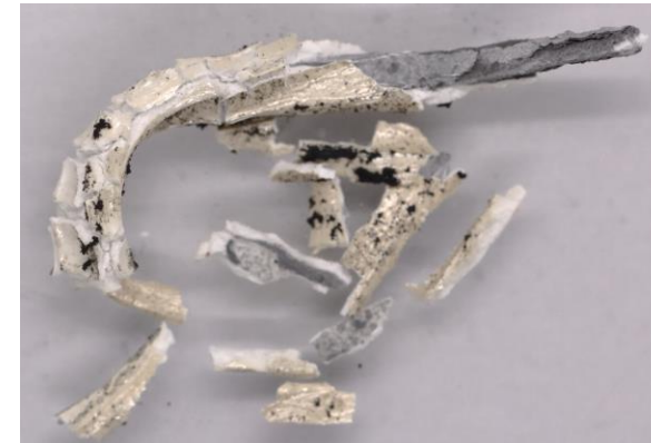
The result of the combined oxidation of a model fuel rod (E110 alloy) and a depleted UO 2 pellet at T=1000°C and conditioning for 3 h
