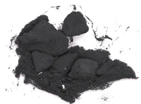
The result of the combined oxidation of a model fuel rod (E110 alloy) and a depleted UO 2 pellet at T=1000°C and conditioning for 3 h
