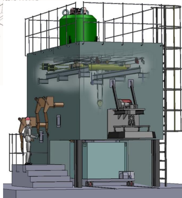
Hot cell for defining RAW characteristics
