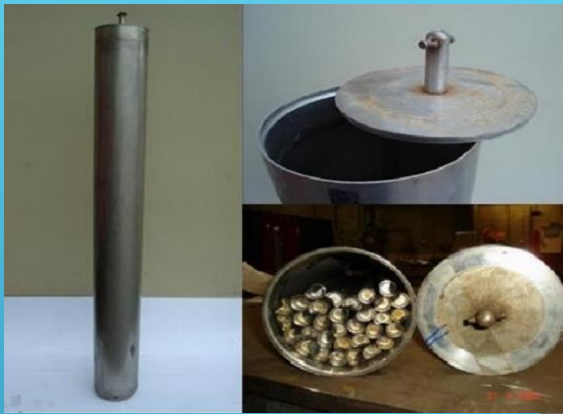
Example of welded can for cut pins/debris
