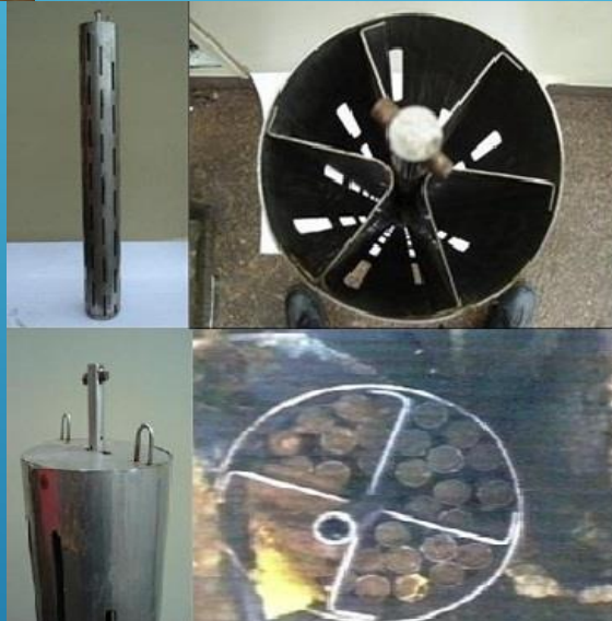
Example of a slotted can for intact pins
