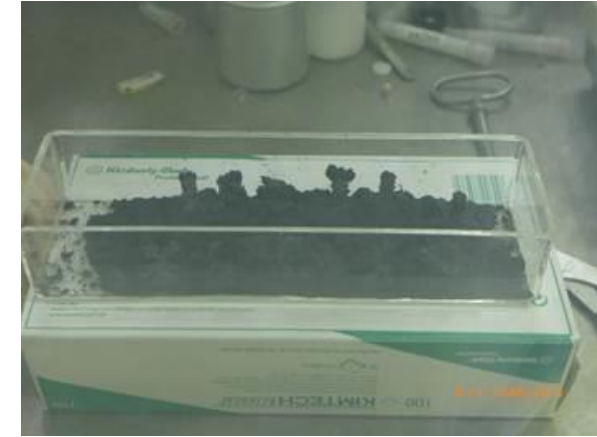
Unirradiated (U,Pu)C pellets (left) and powder produced after oxidation at 800°C (right)
