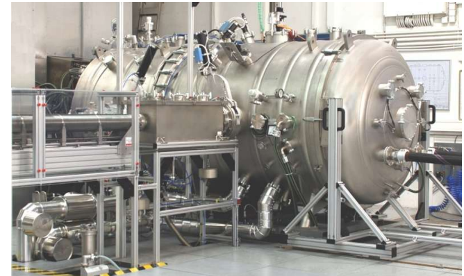
HHF test facility GLADIS @ IPP Garching
