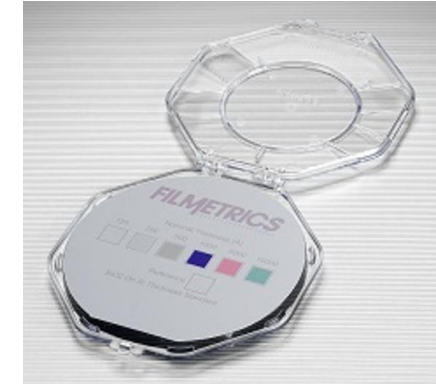
Coating standards ( \text{SiO}_2 on Si)
