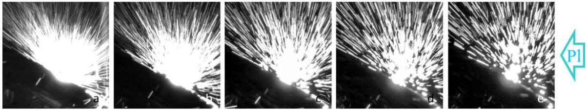
FIG. 6. Images of PSI after a plasma impact on an inclined CPS target (with an incoming plasma energy density of 3 \text{ MJ m}^{-2} ). The images correspond to 1.2-2.4 ms (a); 2.4-3.6 ms (b); 3.6-4.8 ms (c); 4.8-6 ms (d); 6-7.2 ms (e) after the start of the PSI ( t_{\text{exposure}}=1.2 \text{ ms} ).
