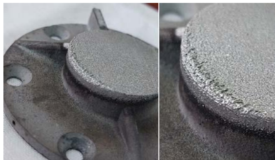
FIG. 7. General view of the CPS target surface exposed to inclined plasma. Images obtained after 50 plasma pulses.
