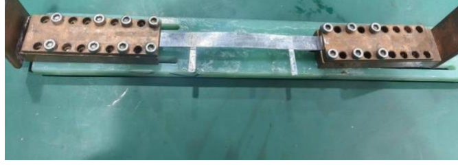
FIG. 15. Physical diagram of critical current testing for stacked superconducting tapes.
