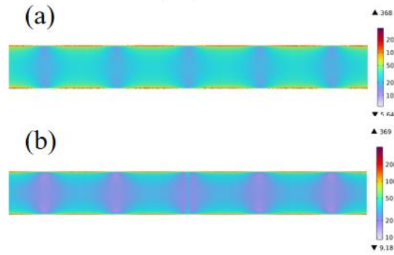
FIG. 8. Stress distribution diagram of two-tape lap joint: (a) Ignoring gap modeling; (b) Not ignoring gap modeling
