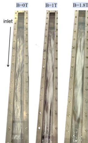
FIG. 4. Film flow pattern under different magnetic field strength (velocity=0.433m/s).
