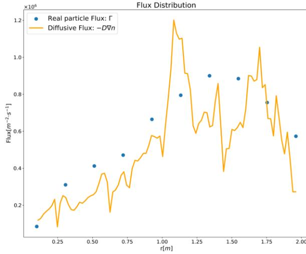
FIG. 6. Comparison of  $\Gamma$  (blue) and  $-D\nabla n$  (orange) along the reduced minor radius  $r$ .
