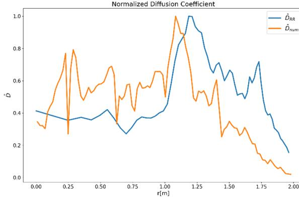
FIG. 7. Comparison of normalized numerical diffusion coefficient  $\hat{D}_{num}$  and the RR diffusion coefficient  $\hat{D}_{RR}$ .
