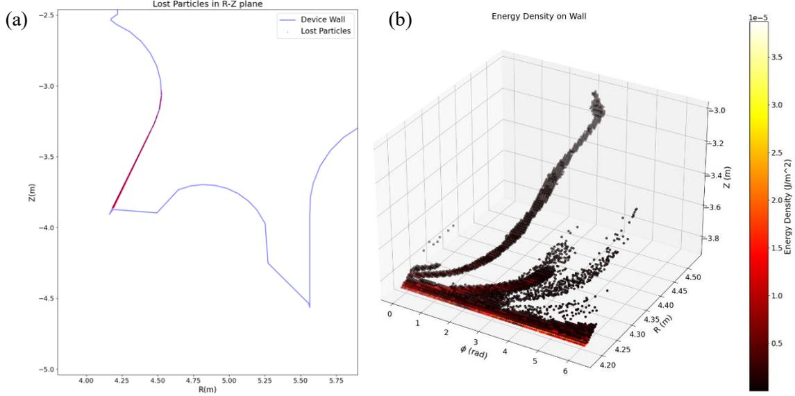
FIG. 5. Lost Position and Heatmap of Lost Energy.
