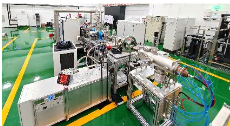
Fig.4 High Intensity D-T Neutron Generator HINEG-II
