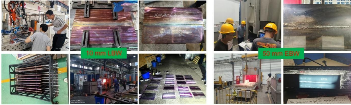
FIG. 6. The different welding methods, process, and properties testing plates of CLAM steel.
