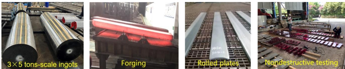
FIG. 5. The 5-ton-scale CLAM steel ingots and corresponding products with different thicknesses.
