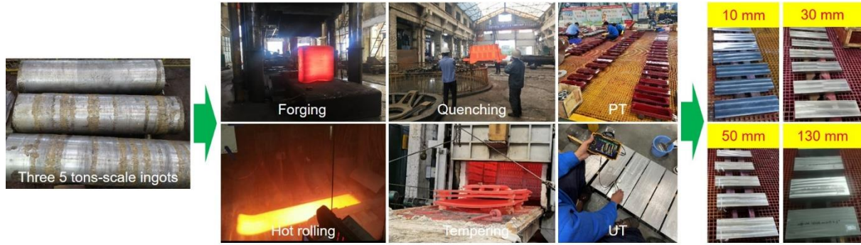
FIG. 2. The 5-ton-scale CLF-1 steel ingots and corresponding products with different thicknesses.
