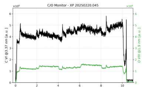
Fig. 2c : Intensity of \text{C}^{5+} (3.4nm) and \text{O}^{7+} (1.9nm) impurity lines as measured by the C/O monitor diagnostic for the discharge of Fig. 2a
