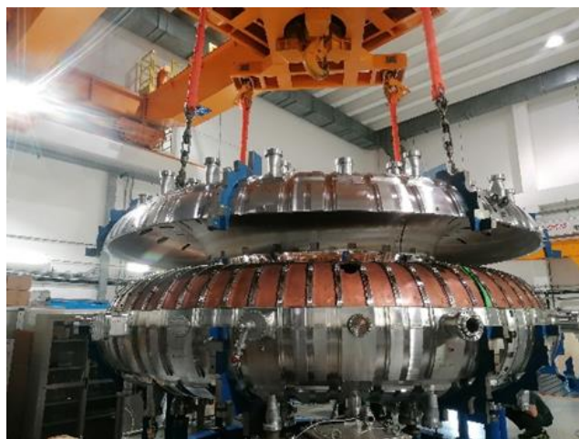
Fig. 1: closing the VTSS with the preliminary assembled PSS inside
