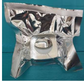
FIG.4. After the cleaning procedure, each ceramic block is placed in a sealed MET-PE bag and vacuumed by the manufacturer.
