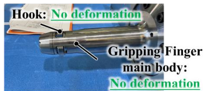
FIG. 6. Confirmation that there are not any deformations in the Gripping Finger after applying the load
