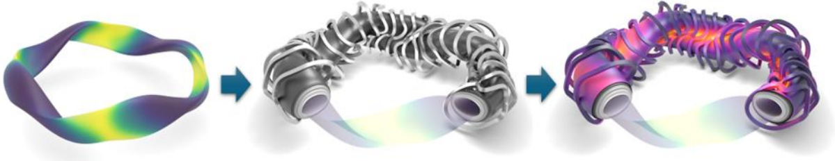
Figure 2: Example workflow starting from a new stellarator magnetic configuration, generating layered blanket structures and performing directly neutron transport simulations on it.
