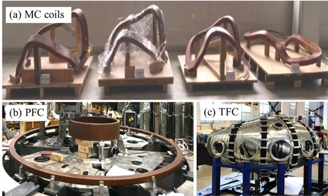
Fig. 5. (a) Photos for the manufactured MC coils, (b) PFC (inner vertical/outer vertical) coils and (c) TFC coils wound on the vacuum vessel surface.
