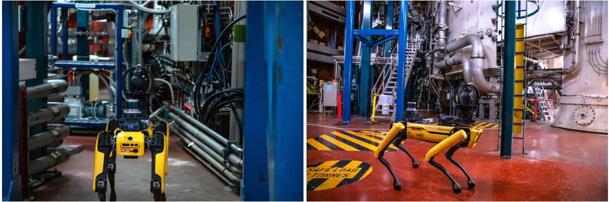
FIG. 8. Long-term autonomous inspection using Spot robot at the Joint European Torus.
