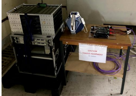
FIG. 4. SEE experiment: test-benches (left and right) and DIAMON neutron spectrometer (center) in JET basement during DTE-3 campaign [10].
