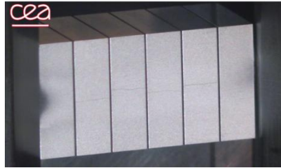
Figure 4 DTT HT mock-up intentionally cracked after 1000 cycles at 16 MW/m 2
