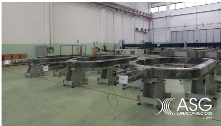
FIG. 1 WP-01, WP-02 and WP-03 maintained in a storage area waiting for the start of their insertion in the casing structure
