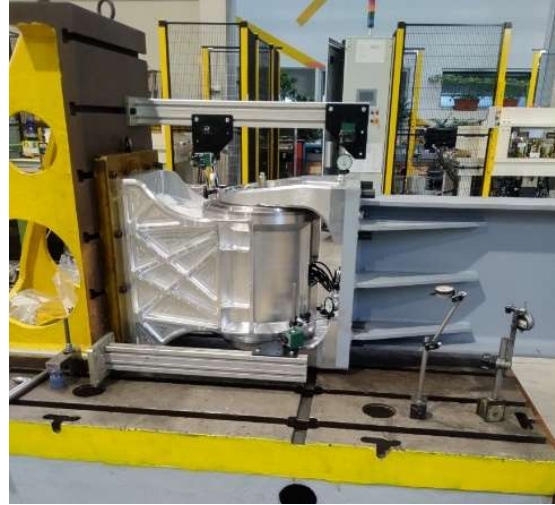
FIG. 6 Image of the Joint # 2 prototype at the qualification tests in OCIMA premises
