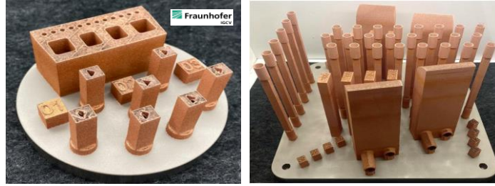
FIG. 2. CuCrZr samples and heat sinks for plasma facing components manufactured using laser powder bed fusion process
