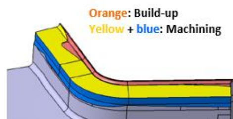
FIG. 10. Illustration of “optimized” repair solution combining build-up and machining
