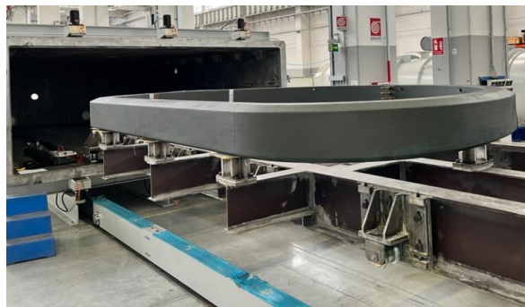
FIG. 4. WP-02 exiting the vacuum chamber after the execution of Paschen test.
