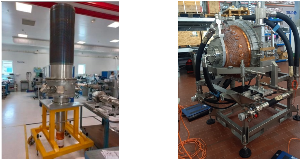
Figure 8. a) DTT first Gyrotron manufactured by THALES. b) RF Load tested in factory.
