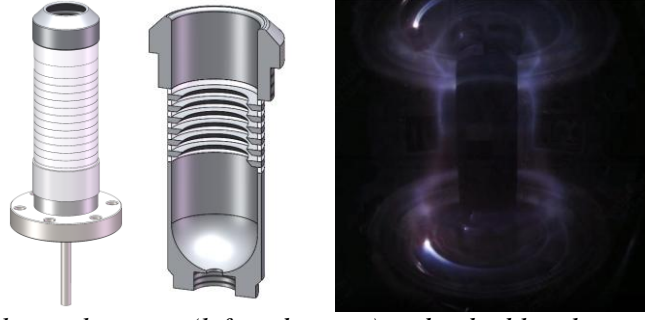
FIG. 3. One design of the washer guns (left and center) and a doublet plasma initiated by dual washer guns for merging (right)
