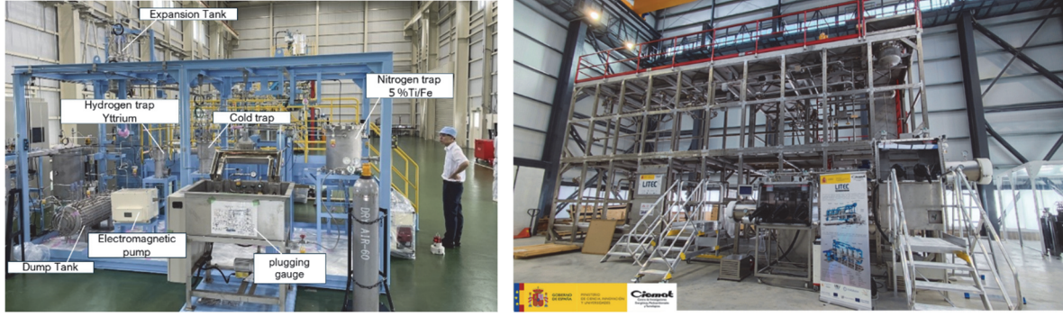
FIG. 11. Lithium loop pilot plants in Japan (left) and in Europe (right)
