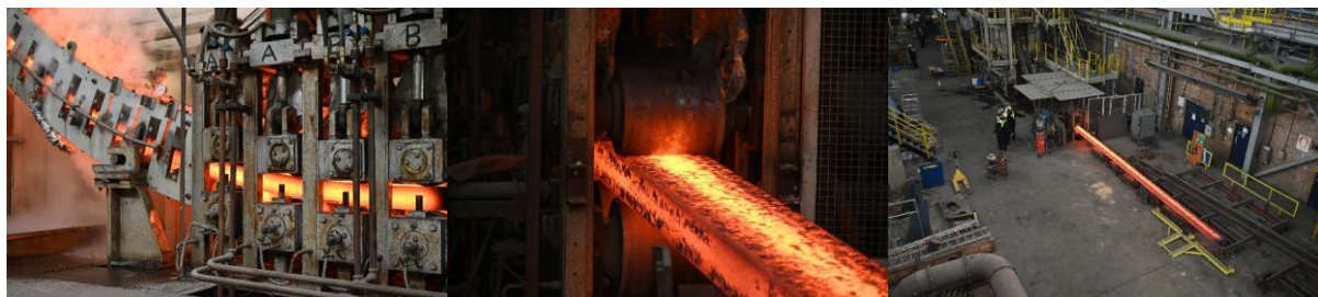
FIG. 10. Fusion grade RAFM steel production at scale in the UK. Continuous casting used to produce an ingot sized at 0.3 \times 0.14 \times 13 metres, weighing approximately 5.5 tonnes [29]
