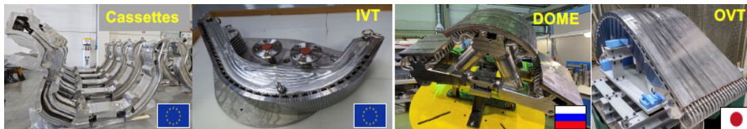
FIG.4. Divertor cassette series production and prototypes of IVT, dome and OVT
