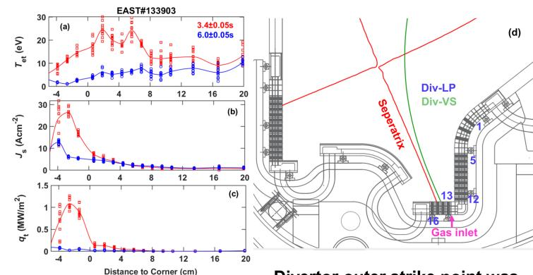
**Profiles measured by divertor Langmuir probes**
