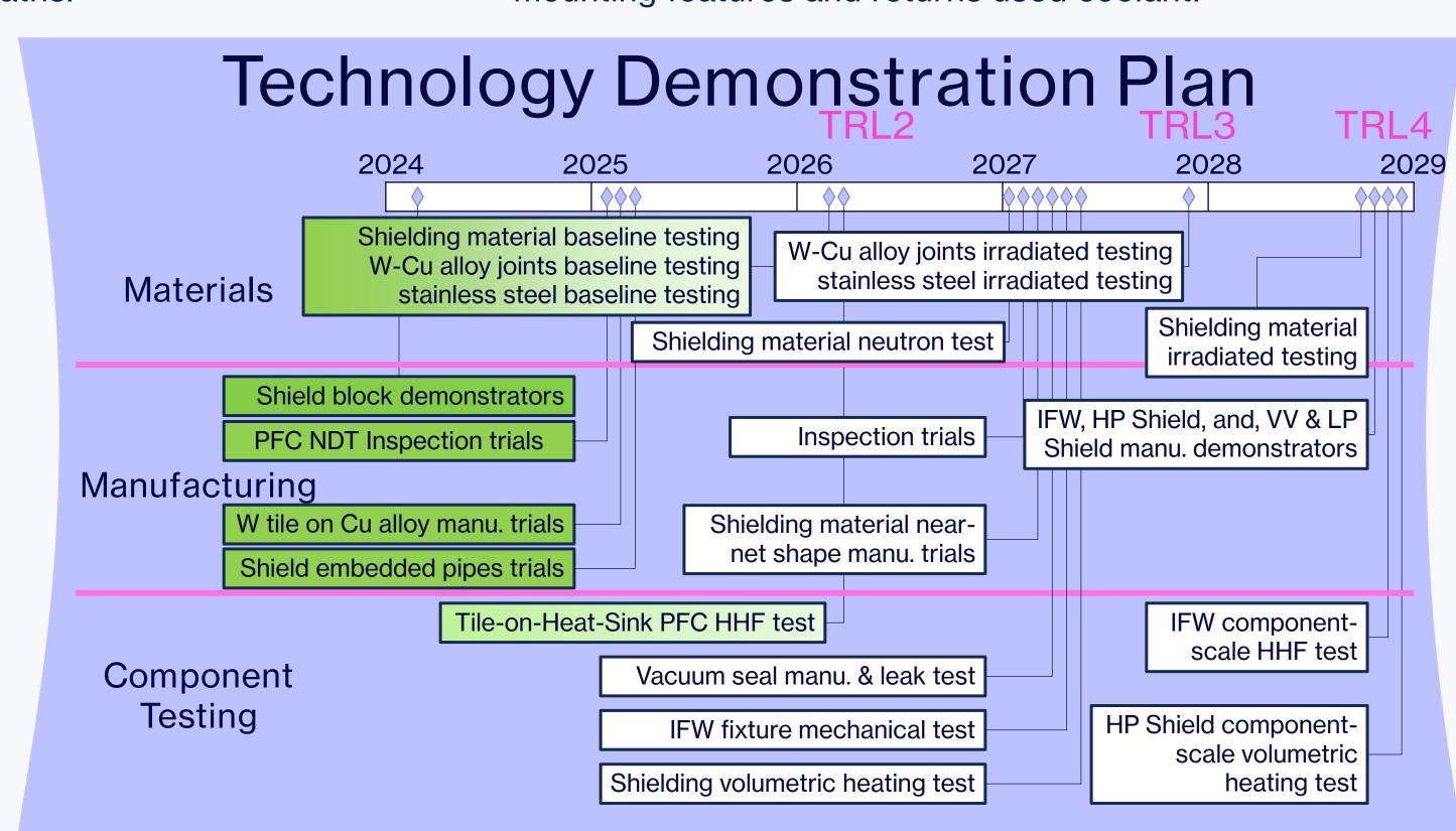
Technology demonstration plan covering the materials, manufacturing and component testing activities for the inboard system with the target of achieving at least Technology Readiness Level (TRL) 4 by 2029.
