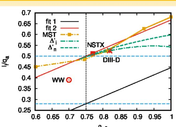
Fit 1: fit of DIII-D database; Fit 2 - eq. (3). "DIII-D" is shot 154576 [Strauss 2023]; "MST" are high  $q_a$  MST, "NSTX" is previous example, dashed lines  $\Delta_i'$ ,  $\Delta_n'$  are marginally stable TMs with ideal and no wall [Strauss 2024], "WW" are TM disruption simulations with highly unstable initialization [White 1977, Waddell 1979], ideal wall. Qualitatively OK, but doesn't fit data. DIII-D and NSTX are rescaled to account for geometry dependence,
