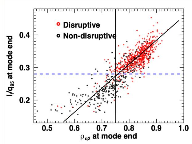
Disruptivity in a DIII-D locked mode disruption database. [Sweeney 2017]. One disruption criterion is  $\rho_{q2}=.75$  or  $q_{75}=2$ .
