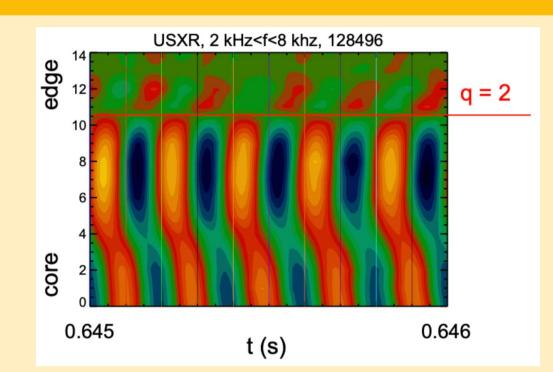
NSTX example with  $\beta_N > 4$ , above the no wall limit. showing soft X ray emission as a function of radius and time. Radial mode structure of feedback stabilized (2,1) mode. It can be identified as a RWTM by its phase inversion at  $\rho_{q2} = 0.75$ . [Sabbagh 2010].
