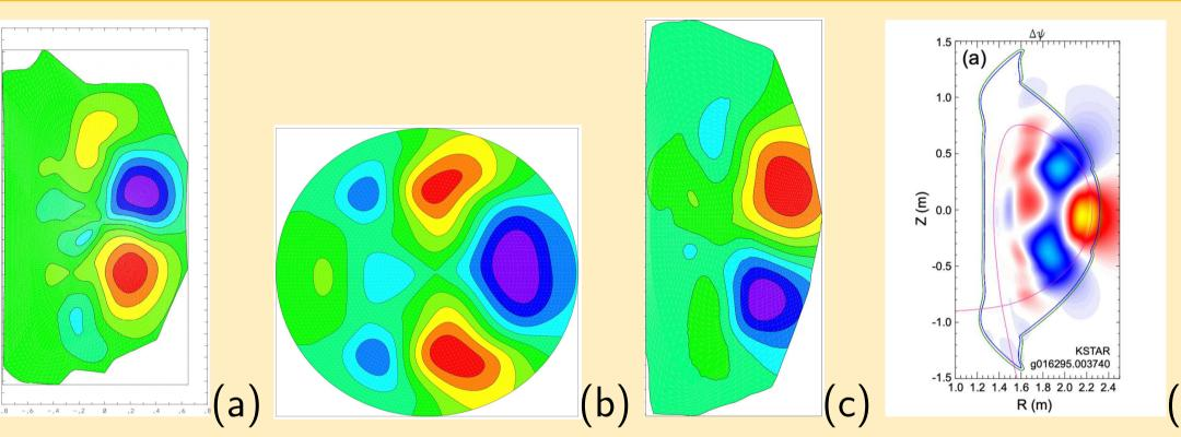
(a) Perturbed  $\psi$  in DIII-D simulations [Strauss 2023], (b) MST - based sequence in Section 4, (c) NSTX in section 8, (d) KSTAR [Y.S. Park 2020].
