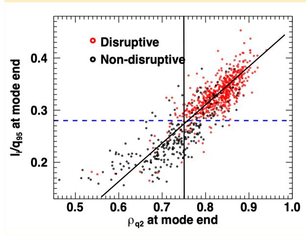
Disruptivity in a DIII-D locked mode disruption database. [Sweeney 2017]. One disruption criterion is  $\rho_{q2}=.75$  or  $q_{75}=2$ .
