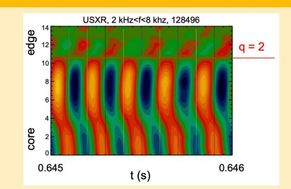
NSTX example with  $\beta_N > 4$ , above the no wall limit. showing soft X ray emission as a function of radius and time. Radial mode structure of feedback stabilized (2,1) mode. It can be identified as a RWTM by its phase inversion at  $\rho_{q2} = 0.75$ . [Sabbagh 2010].
