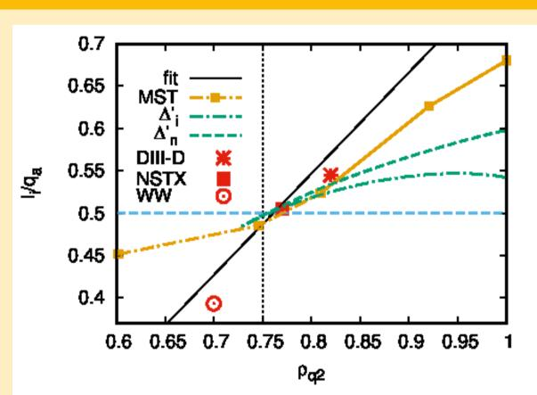
fit of DIII-D database; "DIII-D" is shot 154576 [Strauss 2023]; "MST" are high  $q_a$  MST, "NSTX" is previous example, dashed lines  $\Delta_i'$ ,  $\Delta_n'$  are marginally stable TMs with ideal and no wall [Strauss 2024], "WW" are TM disruption simulations with highly unstable initialization [White 1977, Waddell 1979], ideal wall. Qualitatively OK, but doesn't fit data. DIII-D and NSTX are rescaled to account for geometry dependence,
