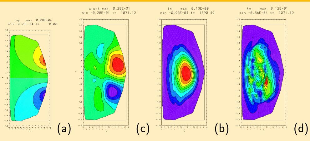
Simulations with modified equilibrium reconstruction of NSTX example [Strauss 2025], with  $\beta_N=3$ . Contours of pressure for NSTX with  $\beta_n=3$  and (a)  $\psi$  produced by feedback coils; (b) pressure contours with feedback; (c) perturbed  $\psi$  without feedback; (d) pressure contours without feedback. Note approximate alignment of (a),(c).
