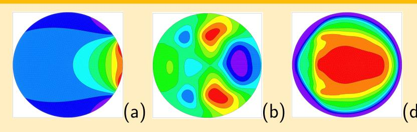
(a) perturbed magnetic flux  $\psi$  from coils (b) perturbed  $\psi$  with resistive wall,  $q_a=3$ . (c) pressure contours with feedback stabilization using the coils.
